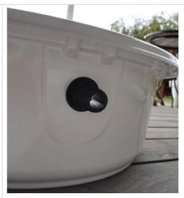
The larger fitting, is for the bigger hole. Mount the sealing from the inside. There is a slightly longer threaded side. Place it to the outside of the base and screw the L on it so it points upwards.
